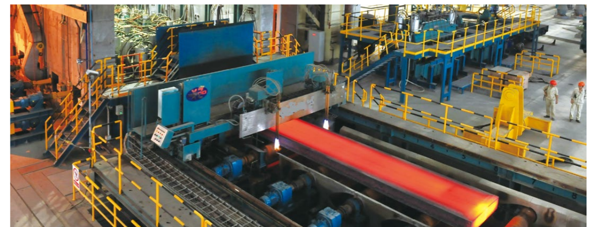
The world's first \geq 450 mm ultra-thick straight-arc slab continuous casting production line
